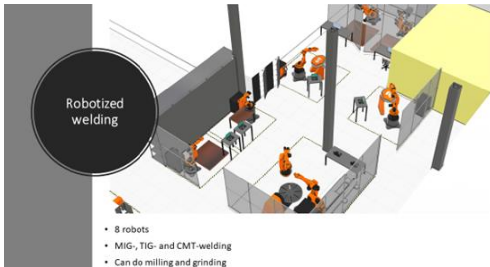
Figure 19: Robots for welding, milling and grinding
